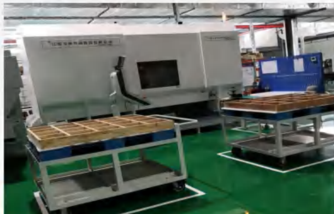
摆线定子数控成型磨床 Wire stator CNC formed grinder 瑞士美盖勒 Mägerle, Switzerland 加工精度达4级 Machining accuracy up to Level 4 价值人民币1670万 Value RMB 16.7 million
