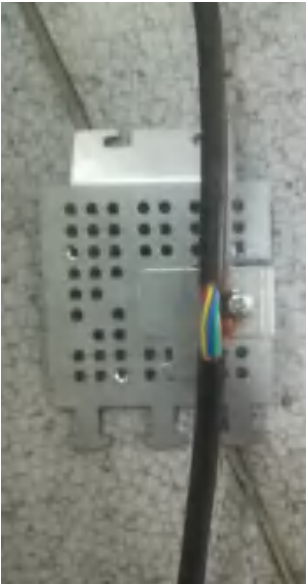
EMC wiring of Power Module B1
